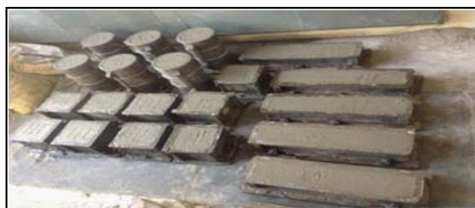
Fig.1: freshly compacted and placed concrete mixes
