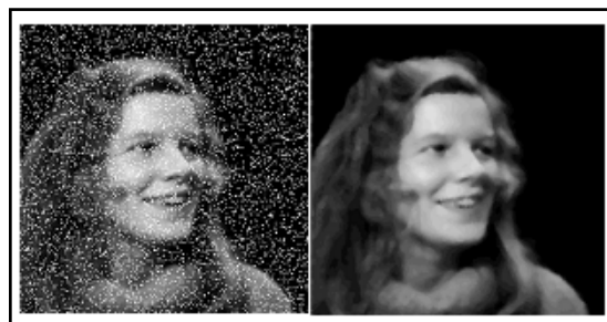
Fig. 1 Noisy image and median filtered image
